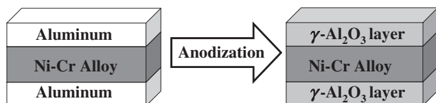
Figure 1. The preparation of anodic alumina supported Ni SRM catalysts.
